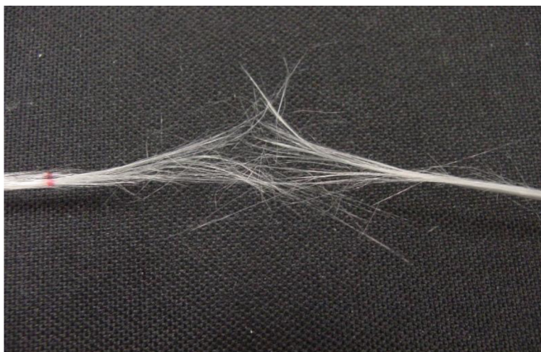
Figure 27. Vectran fiber after AOBF exposure of 1 \times 10^{21} atoms/cm 2 .
