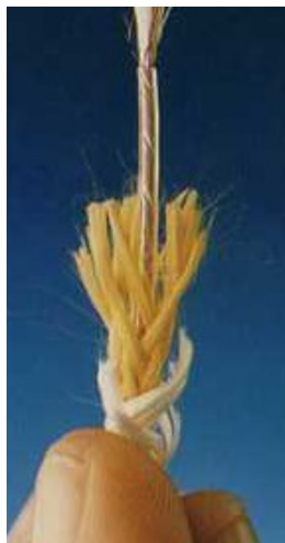
Figure 14. Tethered satellite tether of Nomex outer braid, Kevlar strength fibers, with center core of Nomex and copper wire insulated with Teflon™. 3
