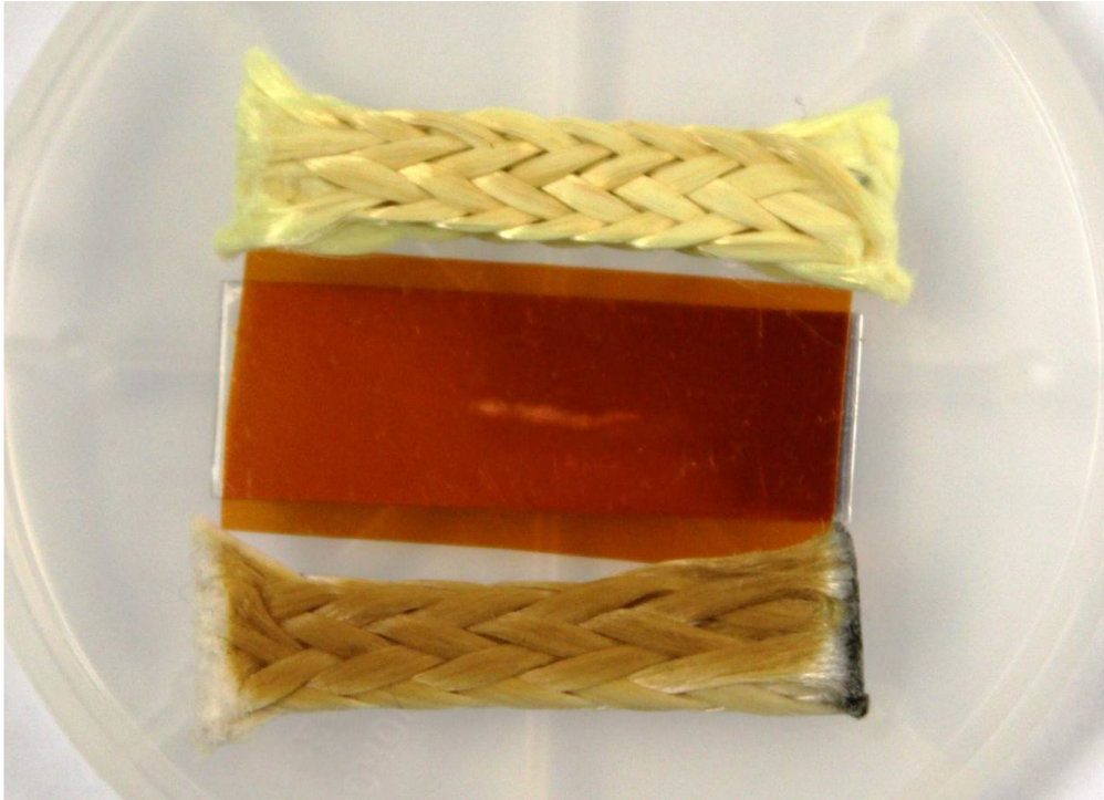
Figure 9. Ram-side Kevlar (top) and Vectran (bottom) cord, postflight, with Kapton witness sample (erosion visible in center).
