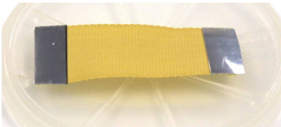
Figure 13. Kevlar strap taped down in empty space between N7-W and N9-W trays, postflight.
