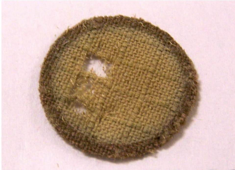
Figure 17. MISSE-2 ram-facing, nonstretch Nomex, sample 2-E8-26, postflight. Significant AO erosion.
